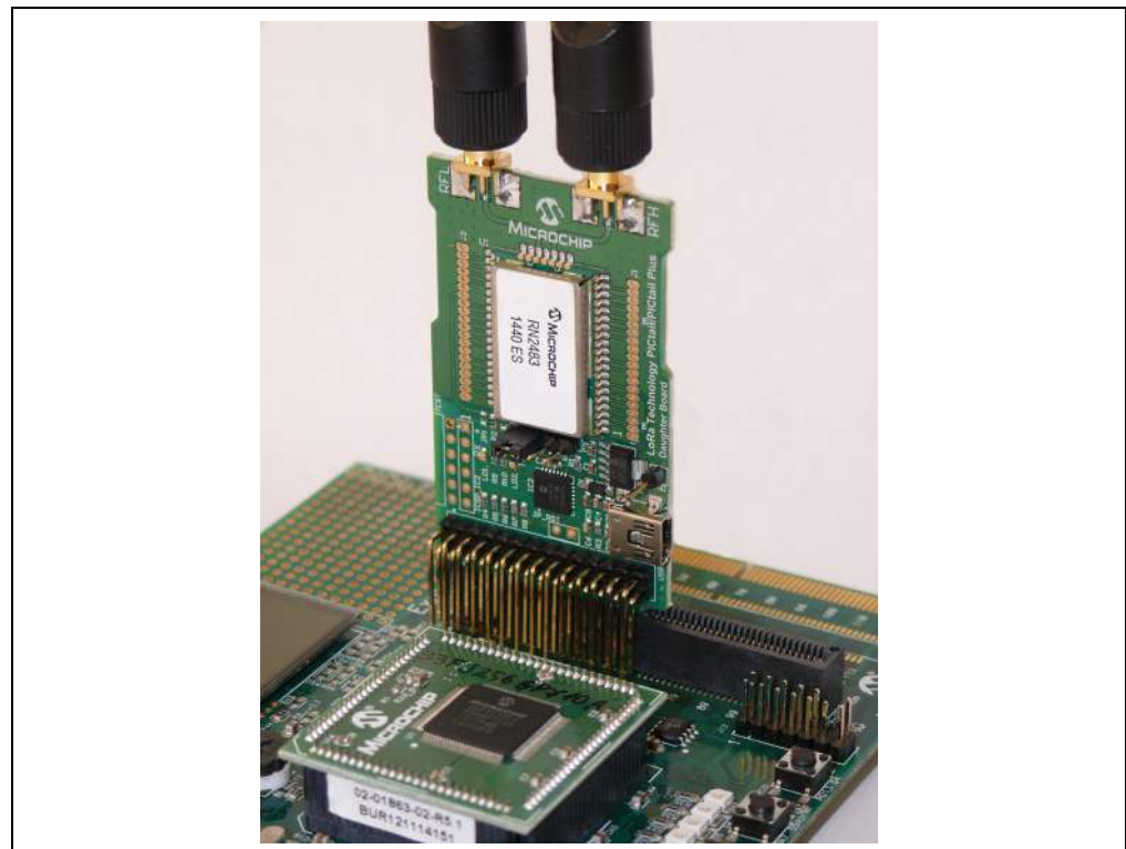
FIGURE 1-2: RN2483 LORA™ TECHNOLOGY PICTail™/PICTail PLUS DAUGHTER BOARD CONNECTED TO EXPLORER 16 DEVELOPMENT BOARD
