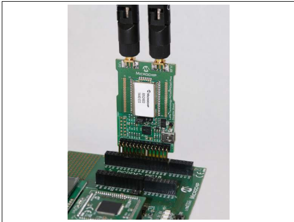
FIGURE 1-4: RN2483 LORA™ TECHNOLOGY PICtail™/PICtail PLUS DAUGHTER BOARD CONNECTED TO PICDEM™ PIC18 EXPLORER DEMONSTRATION BOARD
