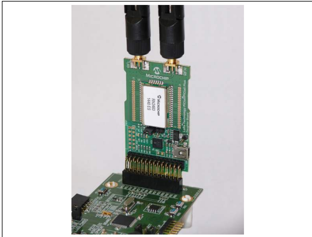
FIGURE 1-3: RN2483 LORA™ TECHNOLOGY PICtail™/PICtail PLUS DAUGHTER BOARD CONNECTED TO PIC18 WIRELESS DEVELOPMENT BOARD
