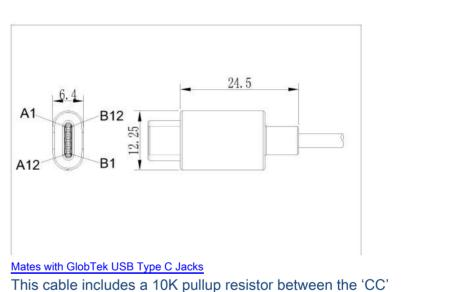
This cable includes a 10K pullup resistor between the 'CC' line and ' $V_{BUS}$ '. For systems compliant with the USB Type-C Cable and Connector Specification, the cable current will be restricted to 3.0A.
