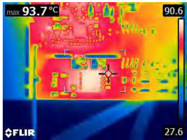
Figure 8-19. V_{IN} = 264 V_{AC} , Bottom-side SR-FET gate-drive R11: 93.7°C
