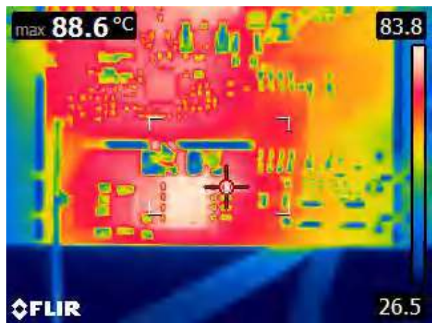
Figure 8-21. V_{IN} = 180 V_{AC} , Bottom-side SR-FET gate-drive R11: 88.6°C
