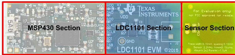
Figure 2-3. EVM Break-Away Sections
