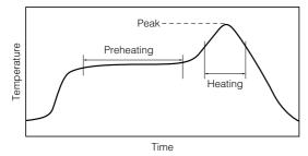
Recommended soldering conditions for flow
