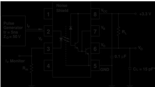
Test Circuit for FOD070L, FOD270L
