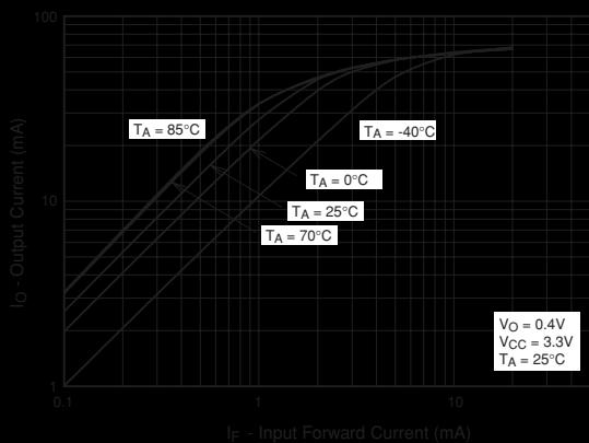
Fig. 9 Output Current vs Input Forward Current (FOD070L only)
