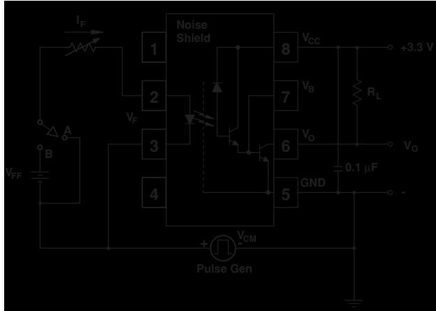
Test Circuit for FOD070L and FOD270L
