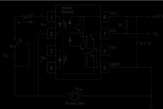
Test Circuit for FOD073L
