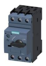
Circuit breaker size S0 for motor protection, CLASS 10 A-release 9...12 A N-release 163 A screw terminal Switching capacity 30 kA at 600 V according to UL/CSA
