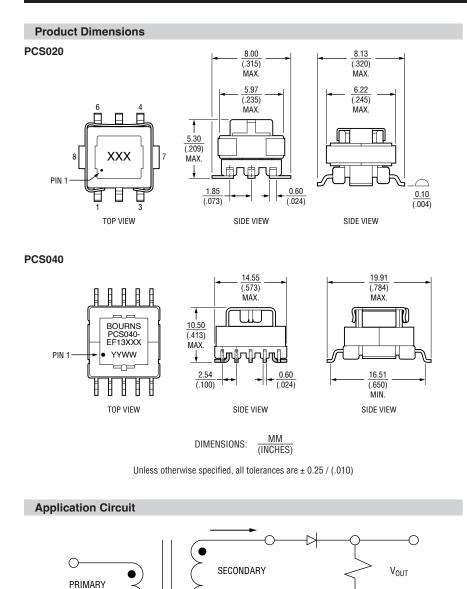
Terminating resistor  ${\sf R}_T$  is based on 1 volt output with the rated current 20 amps for the PCS020 and 40 amps for the PCS040 through the Primary. The terminating resistor can be
