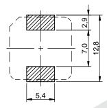
no sensitive traces underneath the component
