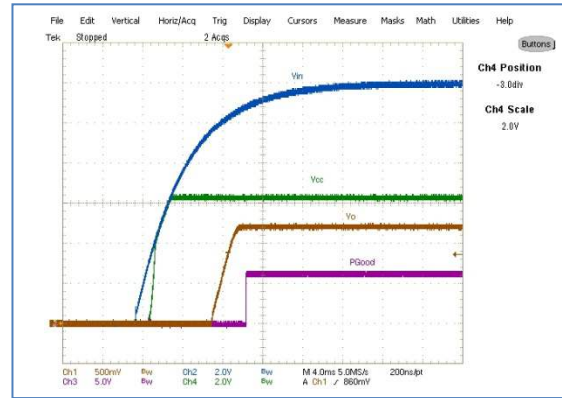
Figure 31: Start up at 16A Load, Ch 1 :V out , Ch 2 :V in , Ch 3 : P Good , Ch 4 : V cc
