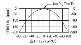
Note: The curve shown above accounts for resonator contribution only and does not include LC component temperature contributions.
