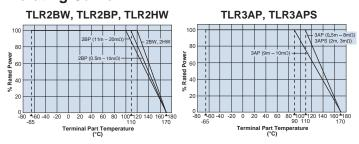
For resistors operated at a terminal part temperature of described for each size or above, a power rating shall be derated in accordance with the derating curve. Please refer to "Introduction of the derating curve based in the terminal part temperature" in the beginning of our catalog before use.
