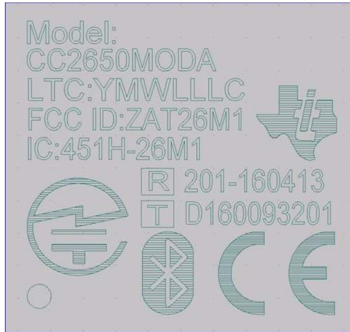
Figure 6-2. SimpleLink CC2650MODA Module Marking
