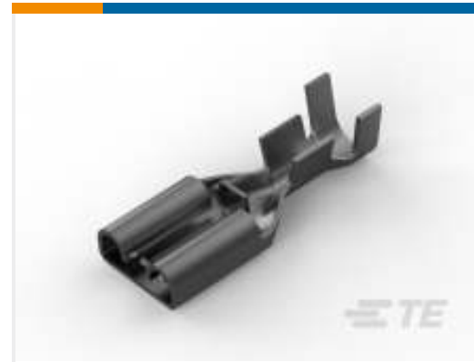
TE Part # 63854-2 250 PL MKIII REC. 18-14AWG TPBR
