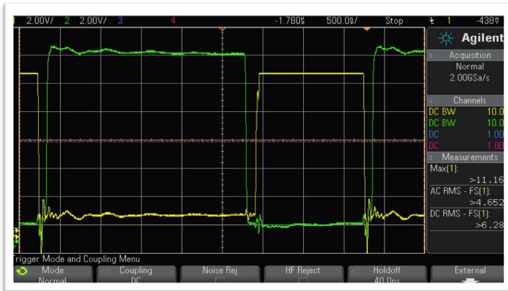
Figure 10: 3.3V/25W Flyback Primary and secondary FETs Gate
