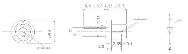
all dimensions in mm. Tolerance  $\pm$  0, 2 except given ones \* at the bottom of the LED
