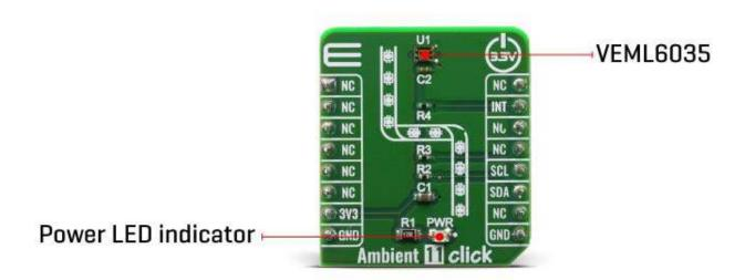
The sensor offers an active interruption feature that is triggered outside of the threshold window settings eliminating loading on the host. Besides that, VEML6035 has excellent temperature compensation to maintain output stability under changing temperature and its refresh rate setting does not need an external RC low pass filter. There is a programmable shutdown mode which reduces current consumption to 0.5  $\mu A$ . Operating voltage ranges from 1.7 V to 3.6 V.
