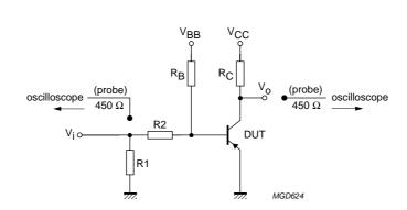
$$\begin{split} V_i = -9.5 \text{ V; T} &= 500 \text{ } \mu\text{s; } t_p = 10 \text{ } \mu\text{s; } t_r = t_f \leq 3 \text{ ns.} \\ R1 &= 68 \text{ } \Omega; \text{ } R2 = 325 \text{ } \Omega; \text{ } R_B = 325 \text{ } \Omega; \text{ } R_C = 160 \text{ } \Omega. \end{split}$$
