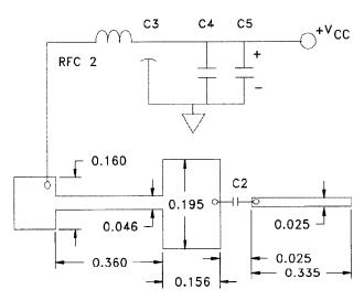
All dimensions are in inches. Substrate material: .025 thick Al<sub>2</sub>O<sub>3</sub>
