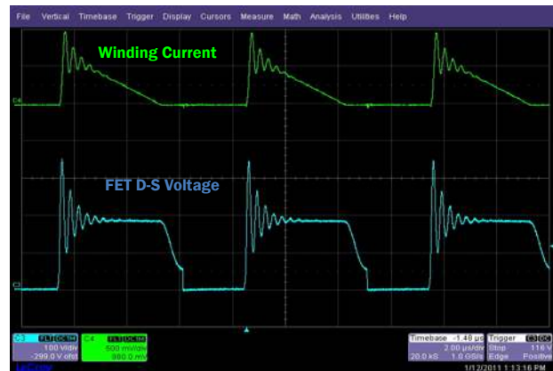
FIGURE 16. QUASI-RESONANT NEAR-ZVS SWITCHING
