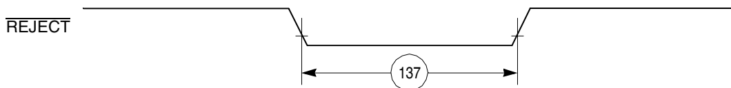
Figure 65. CAM Interface \overline{\text{REJECT}} Timing Diagram
