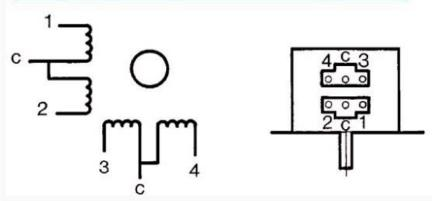
Energisation sequence for clockwise rotation: 2 phases energised (viewed shaft end, front forward) Commons connected to positive.
