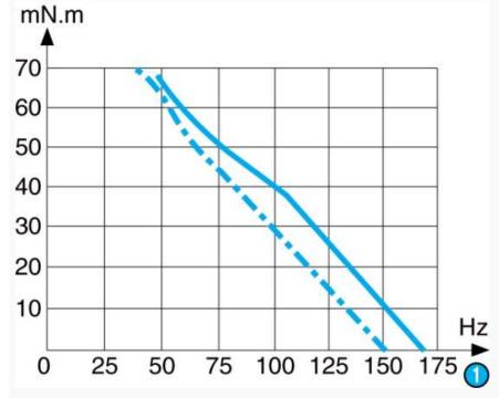
Max. stopping-starting and operating curves at I constant (PBL 3717) for 2 (motor) phases 9 ohms. Holding torque 150 mN.m Current per phase 0.53 A
