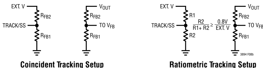
Figure 9(b): Setup for Ratiometric and Coincident Tracking
