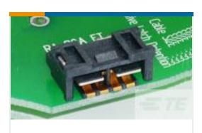
TE Part #1982295-6 ELCON MINI 2P RA HEADER,GOLD,W /O CODING
