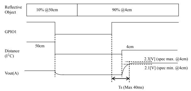
Response time of  $I^2C$  output is faster than that of Vout(A) because it is stabilized soon after distance data output. Distance data is updated every 2ms after response time.
