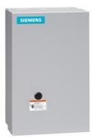
Non-reversing NEMA contactor, Size 4, Three phase full voltage, Contactor amp rating 135A, 3 wire (NO aux included), 110V 50Hz / 120V 60Hz coil, Non-combination type, Enclosure NEMA type 1, Indoor general purpose use, Standard width enclosure
