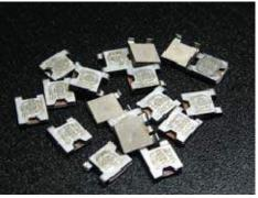
The Zener diode used for voltage clamping in a PolyZen microassembly was selected due to its relatively flat voltage vs current response. This helps improve output voltage clamping, even when input voltage is high and diode currents are large.
