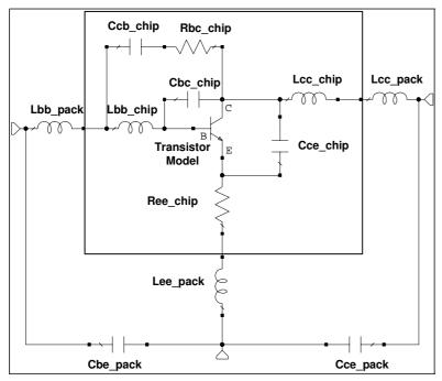
0.212 nΑ  $L_{\text{bb\_chip}} =$ 0.07472  $L_{\rm cc\ chip} =$ nΗ 0.0184 nΗ L<sub>bb</sub> pack = nΗ  $L_{cc}$  pack = 0.277 nΗ 0.239 L<sub>ee pack</sub> = 0.015 рF  $C_{\rm bc\ chip} =$ 0.013 pF  $C_{\text{cb\_chip}} =$ 0.282  $C_{\text{ce chip}} =$ рF 0.064 рF  $C_{\text{be pack}} =$ 0.0492 pF Cce pack = 7 Ω  $R_{\rm bc\ chip} =$ 0.566 Ω  $R_{\text{ee chip}} =$ Valid up to 6GHz
