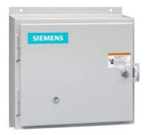
Non-reversing motor starter, Size 0, Single phase full voltage, Solid-state overload relay, OLRelay amp range 3-12a, 24Vdc coil, Non-combination type, Enclosure type 12, Dust/drip proof for indoors, Standard width enclosure
