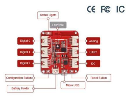
Wio Link is designed to simplify your IoT development. It is an ESP8266 based open-source Wi-Fi development board to create IoT applications by virtualizing plug-n-play modules to RESTful APIs with mobile APPs.
