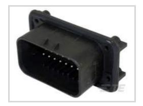
Connector System: Wire-to-Board Number of Positions: 23 Centerline (Pitch): 4 mm [.157 in ] Sealable: Yes PCB Mount Orientation: Right Angle
