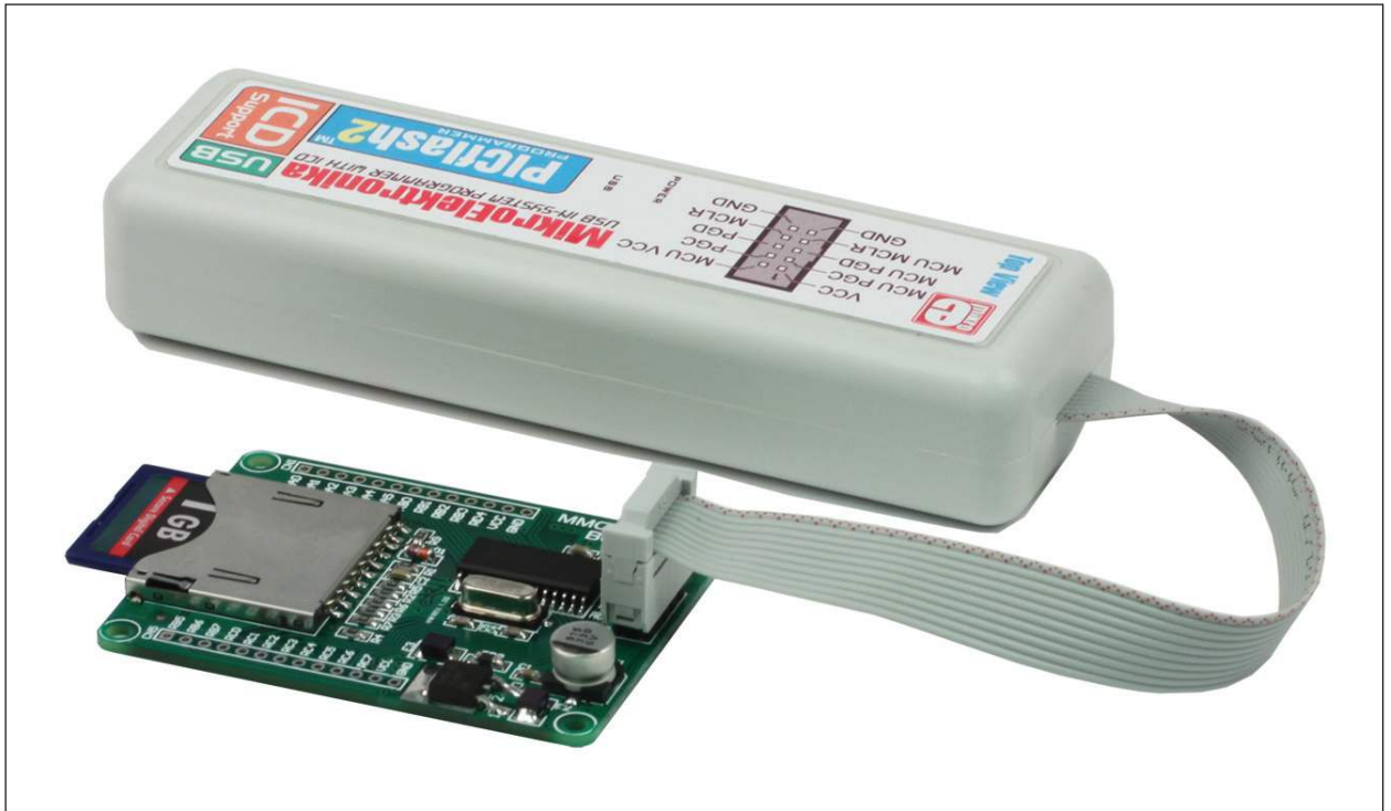
Figure 2: MMC Ready additional board connected to a programmer
