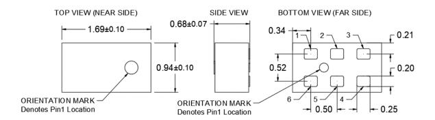
Dimensions are in Millimeters Tolerance are Non-Cumulative
