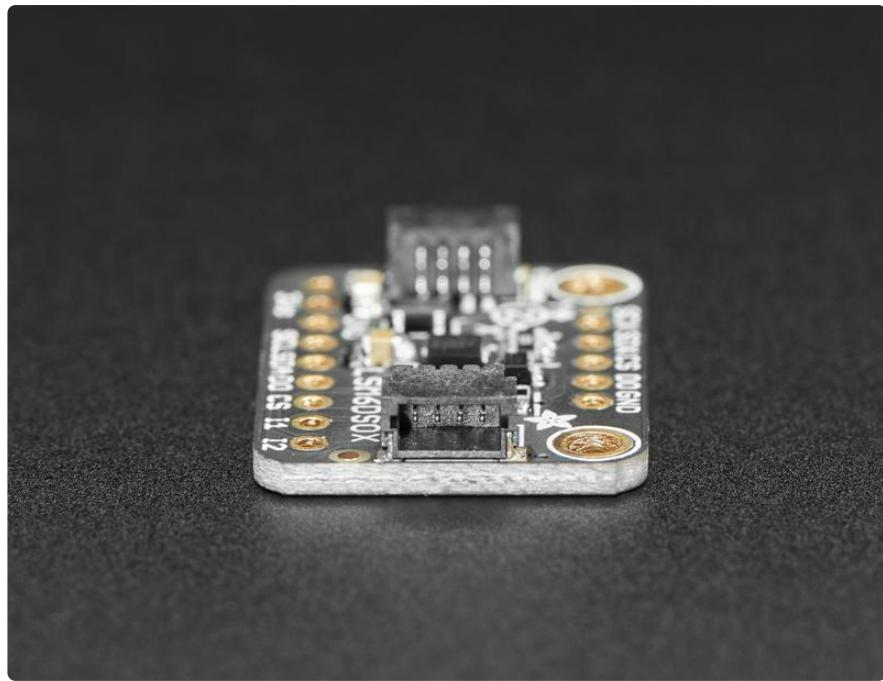
Additionally since it speaks I<sup>2</sup>C you can easily connect it up with two wires (plus power and ground!). We've even included [SparkFun qwiic \(\)](#) compatible [STEMMA QT \(\)](#) connectors for the I<sup>2</sup>C bus so you don't even need to solder! Just wire up to your favorite micro with a plug-and-play cable to get 6 DoF data ASAP.
