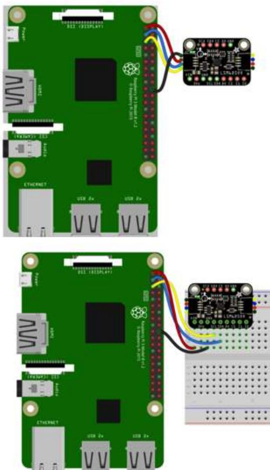
Pi 3V to sensor VCC (red wire)
