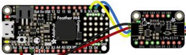
Board 3V to sensor VIN (red wire)
