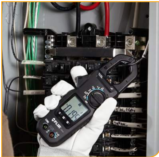
Accu-Tip enables more accurate amperage measurements
