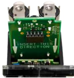
Q45 battery board
