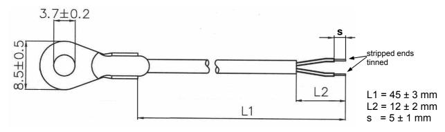
dimensions in mm, tolerances unless specified acc. to DIN ISO 2768-m
