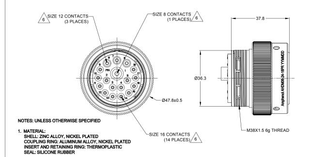
2. MODIFICATIONS: THREADED HOUSING; REDUCED DIA. WIRE SEAL
