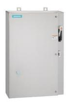
Non-reversing motor starter Size 1 3/4 Three phase full voltage Solid-state overload relay OLRelay amp range 10-40a 110VAC 50HZ / 120VAC 60HZ coil Combination type 60Amp non-fused disconnect Encl NEMA type 4X 316 S-steel Water/dust tight non-corrosive Extra-wide enclosure
