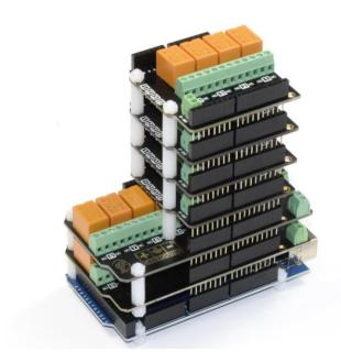
**CANADUINO® Stackable Relay Shield for Arduino** is available as DIY soldering kit with all SMD parts already assembled and trough-hole parts included for DIY assembling.
