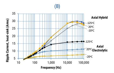
Frequency dependencies of ESR measured at 20oC and 100 kHz for Axial Hybrid (PHA225MKP3370QE4) and Axial Electrolytic (PEG226MG3370QE1) capacitors (A); Frequency dependencies of max. short pulse Ripple Current at different temperatures for heat-sink mounted Axial Hybrid (PHA225MKP3370QE4) and Axial Electrolytic (PEG226MG3370QE1) capacitors (B).
