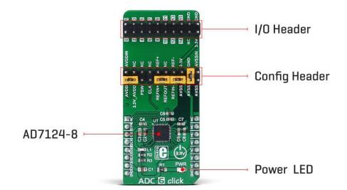
The signal routing in the AD7124-8 ADC is done via the internal multiplexer section, which is used to reduce the number of IC pins, yet allowing all of the functions to be used on the existing pins. On a top of these pins, there are four more GPIO pins that can be used for various tasks, including control of the multiplexer unit. Since the multiplexer is integrated into the chip, the conversion process stays synchronized with the changes made to the pin configuration.
