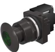
30mm BlackMax, Epoxy Coated Corrosion Resistant Complete Metal Unit Illuminated Push-Pull Operator Full Voltage, 24V AC/DC Incandescent Lamp Mushroom Head Cap Small 1 3/4" (44.5 mm) Metal, Black with Green Lens 2 Position Maintained, Pull-to-Release UL Listed, CSA Certified NEMA 1,3,3R,4,4X,12,13 & Automotive Standards
