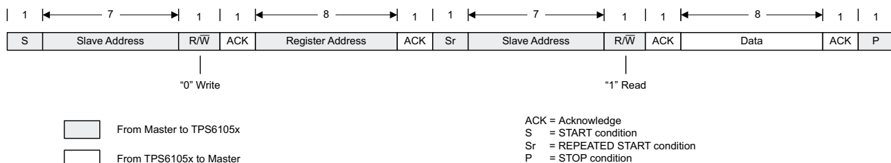
Figure 34. Read Data Transfer Format In F/S-Mode
