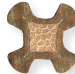
Indenter Crimp Cross-Section Across Axis
