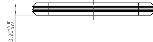
Recommended Waterproof Gasket Gasket Part No.: USBTJ-02 (Gasket must be ordered separately) (See separate datasheet for specification)
