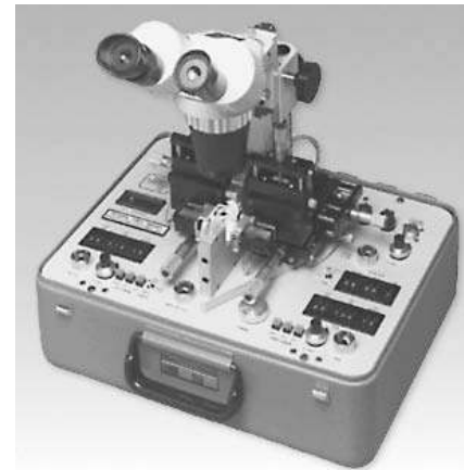
Photo 20. Fusion splice for glass optical fiber.
