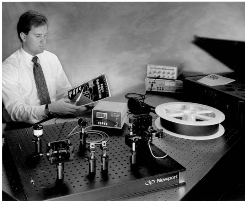
Photo 13. Engineer preparing to measure the attenuation through a spool of optical fiber. (Photo furnished by Newport Corporation.)
