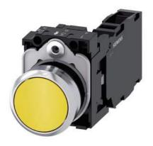
Pushbutton, 22 mm, round, metal, shiny, yellow, pushbutton, flat, momentary contact type, with holder, 1 NO+1 NC, screw terminal
