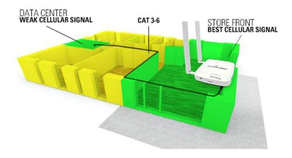
6310-DX can be located to capture the strongest cellular signal strength.
