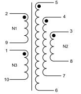
N2 denotes three windings connected in parallel. Terminals 3+4+5 and 6+7+8 must be tied as solder bridging is allowed.
